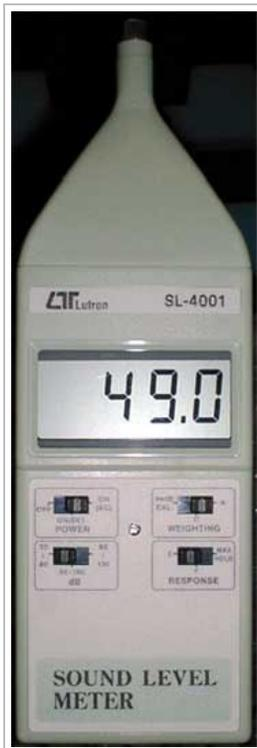
With this measuring device we determined the noise level (dBA) of all coolers.
