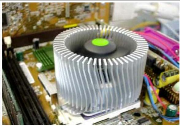
Bad example -the Thermaltake Aircooler looks interesting but does not reach any high cooling effect. There is too much distance between the fins and the processor.
