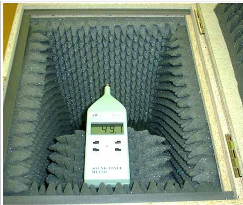
Our miniature sound chamber has enough space for a motherboard, hard disk or even a CPU cooler. The noise level is determined in the middle above the CPU cooler at a constant distance.
