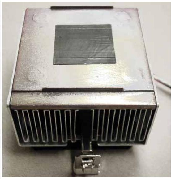
Well designed: Elan Vital's cooler is equipped with a copper heat spreader. In addition to that, it has cooling foils made of aluminum.
